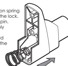
Once the cylinder assembly is in place (in the un-locked position) and the compression spring is inside the lock, the back plate is placed over the spring & retainer pin. Screw on with 3 x BSW screws. The back plate also secures the insert in place.
