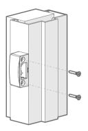
3. Place strike onto strike mounting plate and slide sidewards into position.
