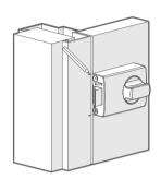
1. Close the door and using the lock case as a guide, mark the position to install the strike on the metal jamb.
